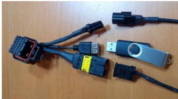
It can be used as it is in a modern car (after 2007 approximately) for rallies "New Energy", learning or reconnaissance before rally. For an older vehicle, it is necessary to add a power supply and a GPS (not very precise) or an interface for sensor (s) wheel
