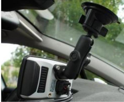
The suction cup can be replaced by a fastening on the dashboard so as not to interfere with the pilot's vision.
